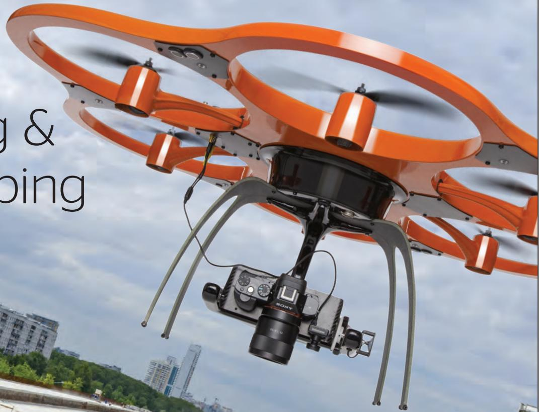
With the **Aibot X6**, you can generate data for orthophotos, 3D models, and point clouds in **high density with great accuracy**. Flight planning software makes it simple to obtain **photogrammetry**, all while **saving time and money!**
